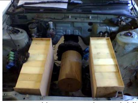
The motor and battery mockups trial-fitting.
