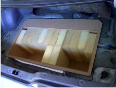
Trial fitting a mockup of the rear battery pack.
