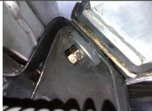
Custom rubber mount secured to original engine mount.
