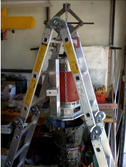
Aligning motor adaptor and gearbox.
