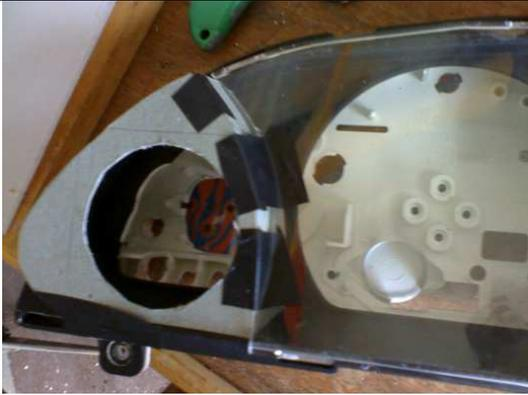
Mocking up the instrument panel mod for the energy meter.
