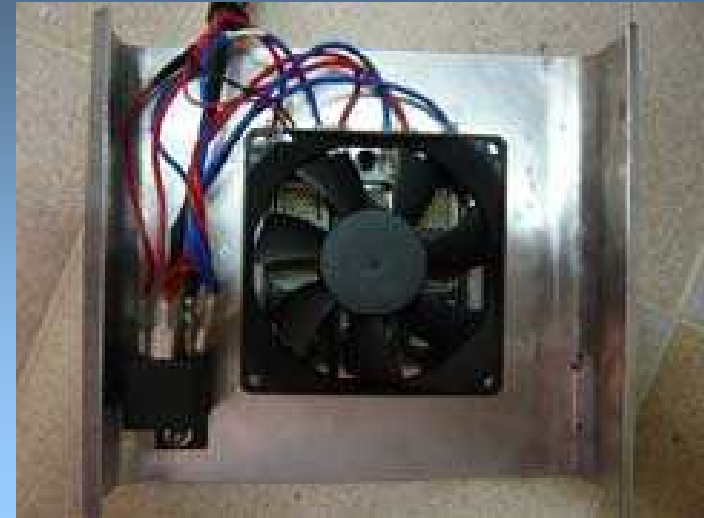
HEATER INSTALLED IN ALUM HOLDER TO ADAPT TO OLD HEATER CORE SPACE
