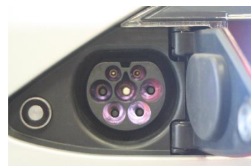
Pic: Tesla modified Type 2 socket (note notch at top to prevent use of Tesla Superchargers with normal Type 2 sockets). Source: Wikipedia
